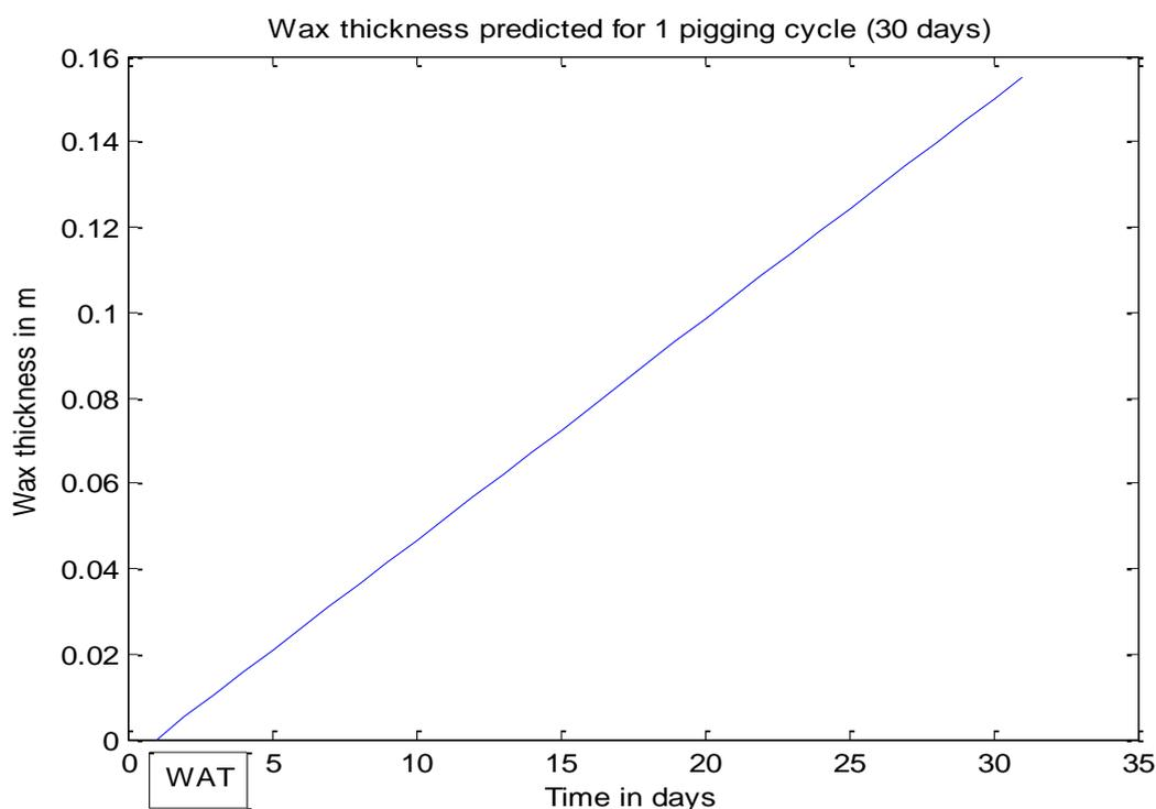
**Fig 6. Wax deposition thickness for 30 days (1 Pigging cycle)**
