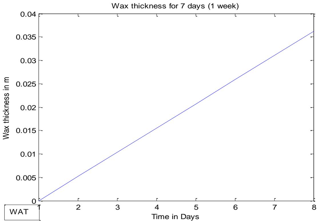
Fig 4. Wax deposition thickness for 1 week (7 days)
