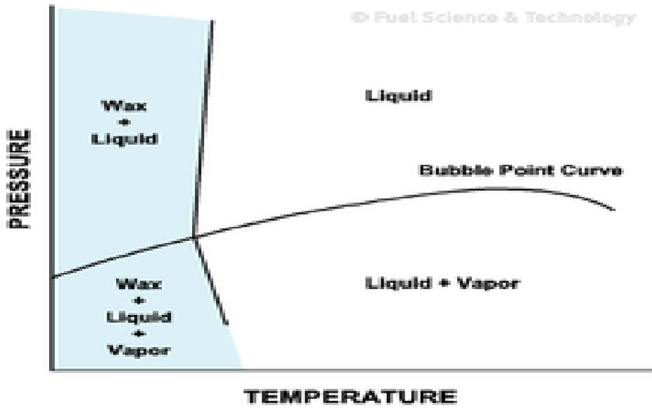
Fig 1. Wax Precipitation Curve (Courtesy: Fuel science and Technology)
